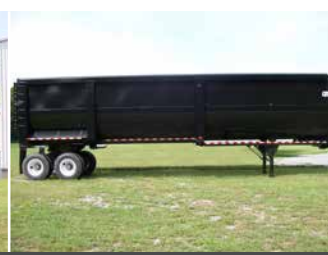
Frameless full width draft arms. All wheels stay on ground
